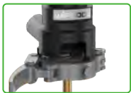
Open the clamp & insert the copper tube
