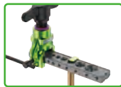
The copper pipe enters the hole, and the limit plate is on the copper pipe
