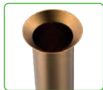
Finalize of expanding 45° copper pipe
