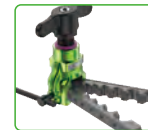
The expansion strip is inserted into the expansion body
